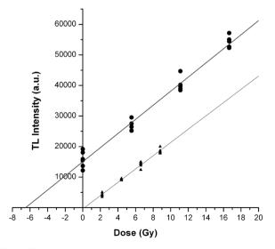
**Fig. 1.** Equivalent beta dose determination by added dose technique of the STS\_TL#4 sample:  $Q_{\beta}$  (circles) and  $q_{\beta}$  (triangles) evaluation from growth curves.
