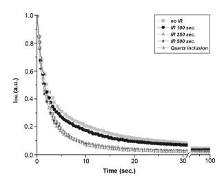
**Fig. 3.** The [post-IR] OSL decay curves for the data shown in Fig. 2 related to STS\_TL#4 sample. The OSL decay curves from FG\* and from QI fraction are compared for IR stimulation times from 0 to 500 s.
