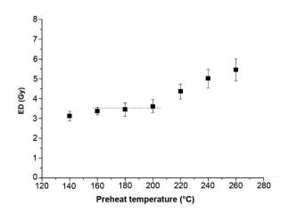
**Fig. 5.** ED values (1σ deviation) obtained on QI-OSL-SAR subsample for STS\_TL#4 sample as a function of preheating temperature. The dotted line shows the ED plateau region.
