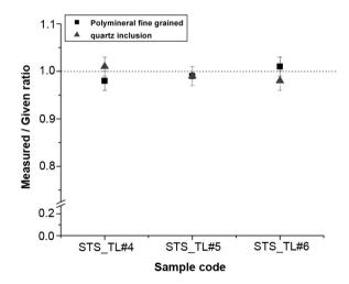
**Fig. 6.** Data obtained from dose recovery test (measured to given dose ratio) on the three analyzed samples (1σ deviation). In the dSAR (FG\*-OSL-dSAR) and SAR (QI-OSL-SAR) sequences, a preheat at 200°C for 10 s and at 180°C for 10 s, were respectively performed both with a cut heat at 160°C.
