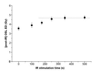
**Fig. 2.** Post-IR OSL ED values for FG fraction of STS\_TL#4 sample, determined for different IR stimulation times after a preheating of 200°C for 10 s. Each point is the average result from three aliquots (1σ deviation), and the corresponding error is calculated using Analyst version 3.24 (Duller, 2007). The dotted line is the mean of the data points from 250 s to 500 s.
