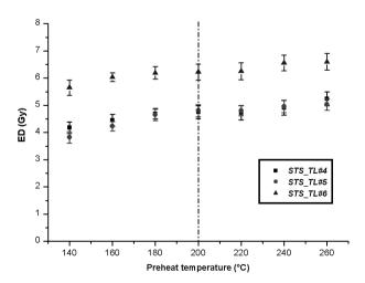
**Fig. 4.** ED values (1σ deviation) obtained on FG\*-OSL-dSAR subsample for STS\_TL#4, STS\_TL#5 and STS\_TL#6 samples as a function of preheating temperature.
